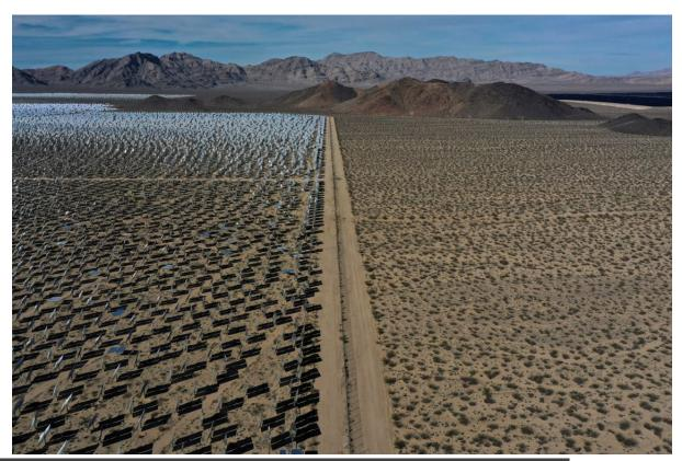
Fields of directed heliostat mirrors are seen at the Ivanpah Solar Electric Generating System (left), and photovoltaic solar panels are seen at the Desert Stateline Solar Facility (far right) near Nipton, California U.S., February 27, 2022. REUTERS/Bing Guan/File Photo
