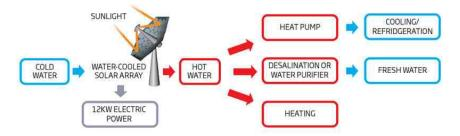
Each panel holds 25 photovoltaic chips cooled by water flowing in microchannels undermeath. These carry the heat away at a rate that leaves the microchips at their optimal operating temperature. That makes the Sunflower more efficient than existing photovoltaic concentrating generators, so it needs a quarter of the panels to produce the same power. This makes it far cheaper, says Michel.
